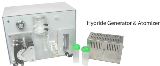
This system comes complete with an advanced gas-liquid separator which allows users to add a drying agent. By removing moisture, pressure fluctuations are minimized, thus enhancing the precision of measurements. Three mixing levels in the reaction/mixing manifold enable the convenient online addition of reagents required for acidity adjustments, pre-reduction/oxidation or masking of interferences.
